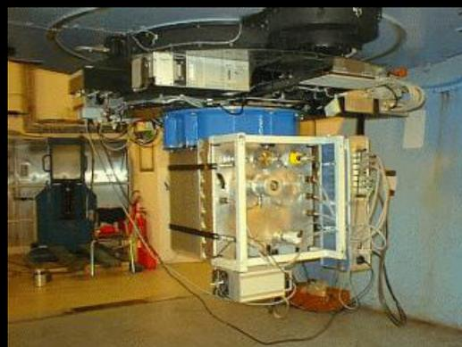
NOTCam (Nordic Optical Telescope infrared Camera and Spectrograph)
