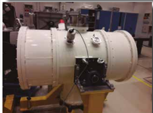
Tenerife Microwave Spectrometer (10-20GHz). Top: 4K cold load (November 2020). Bottom: cryostat in the IAV room at the IAC.
