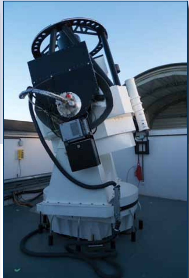
Fig. 3 STELLA-I with WiFSIP and the new CCD camera while doing sky flat fields.
