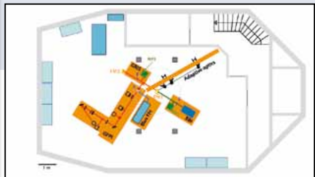
Fig. 3: Top view of the observing room. The beam coming from the adaptive optics bench can be redirected to different optical tables via the rotating fold mirror FM1. FM2 reflects the light to the infrared grating spectrograph that is located one floor below.
