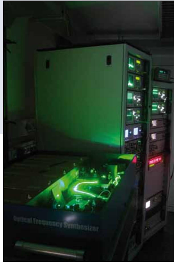
Fig 1: The VTT frequency comb system in operation. Laser and optical components are contained in the blue box in the foreground. The two racks in the background contain the control electronics and monitoring systems. The light from the laser is fed to the spectrograph in an optical single mode fiber.
