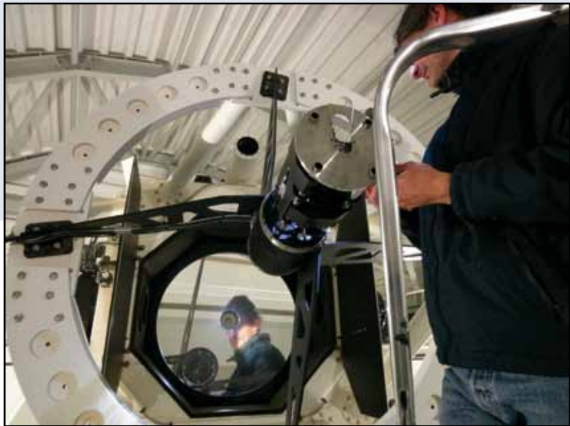
Fig. 1: Work being carried out on STELLA-II's prime-focus fibre-feed unit.
