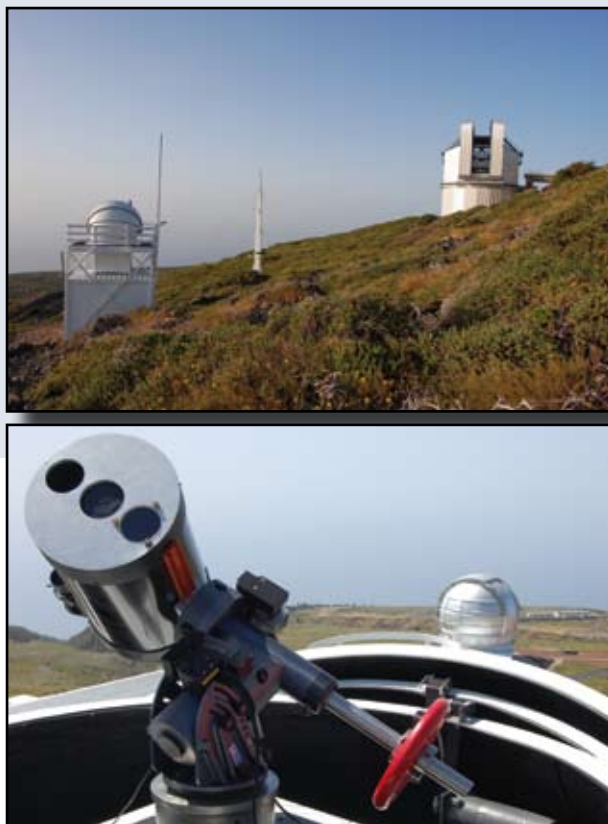
Figure 3: Two images of the TNG-DIMM. (a) The tower and the dome that houses it with the TNG in the background. (b) The TNG-DIMM with Grantecan in the background.
