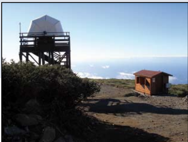
Figure 1: Weather station at Las Moradas (ORM), consisting of a MASS-DIMM on a 5m high tower (left) and a weather station with standard weather sensors (right).
