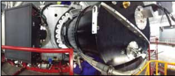
Fig. 1: the near-infrared camera CIRCE, which is a visitor instrument built at the University of Florida.
