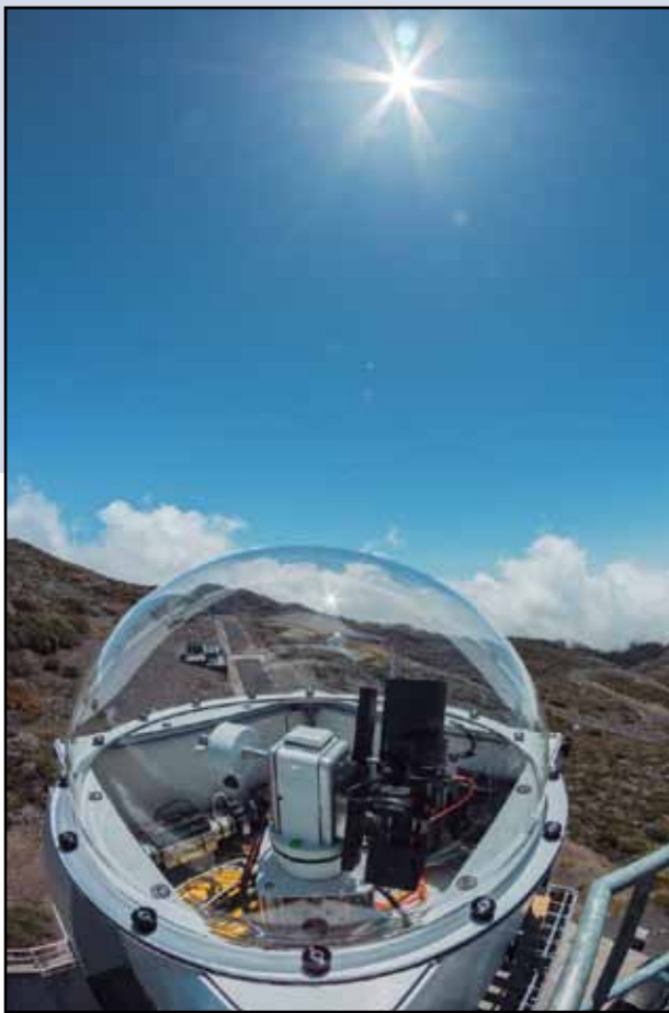
Fig. 1: The solar telescope consists of a 7.6 cm diameter lens focusing the full disk of the Sun into an integrating sphere which feeds the calibration system of HARPS-N. The telescope tracks the Sun while the HARPS-N spectrograph acquires spectra every five minutes.
